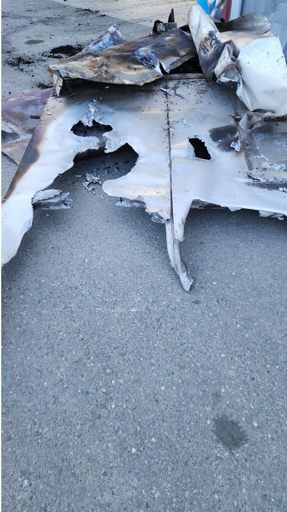
Figure 2: Vault Door w/Melted Aluminum Sheet
