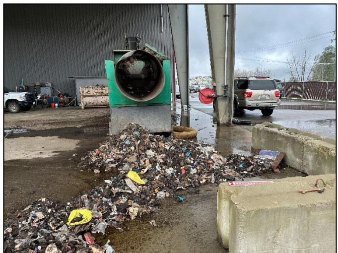
Figure 56 - Debris screened from finished compost material.
