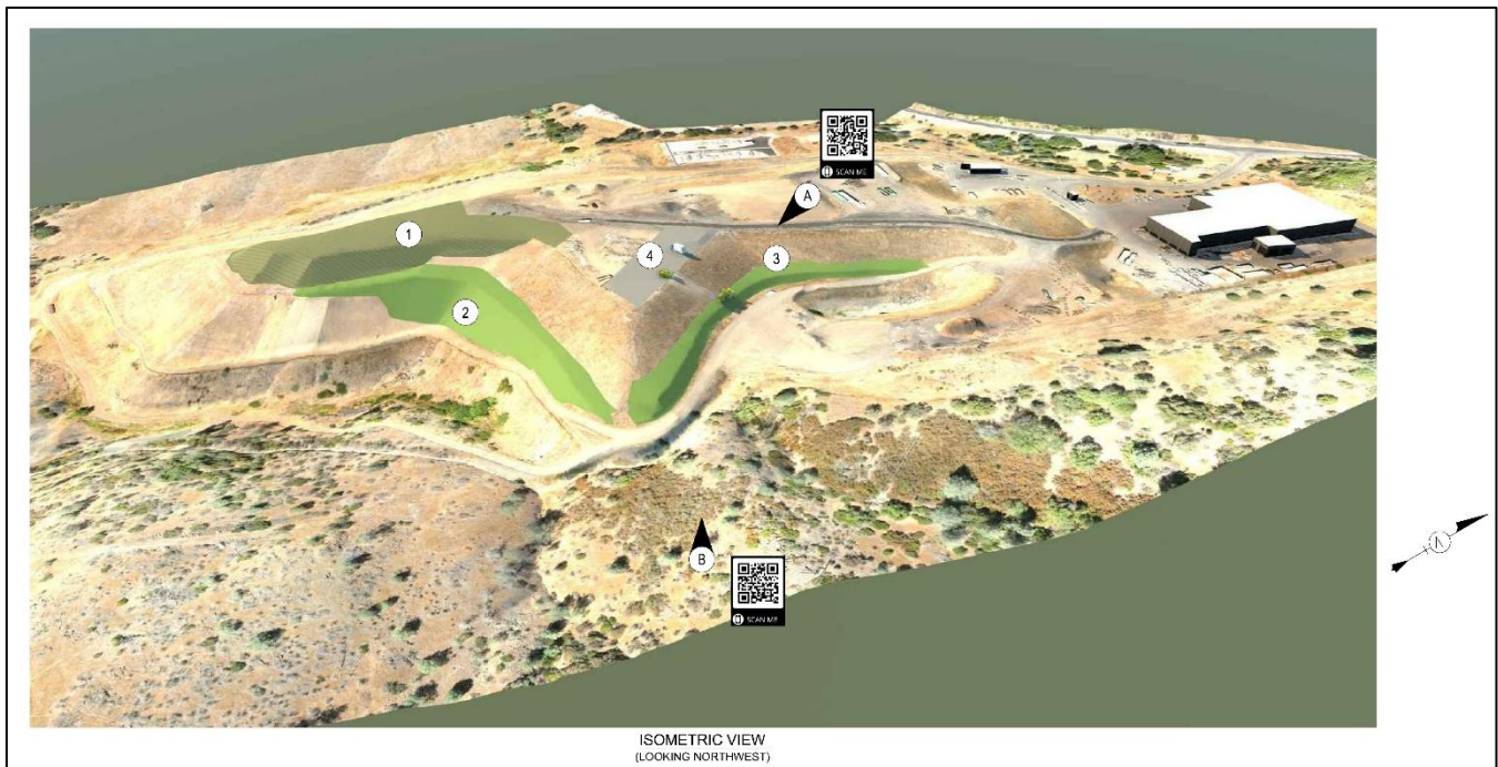
Figure 54 - Isometric view of proposed fill locations from 2020 Fill Sequence Plans.
